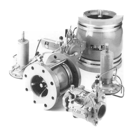
The Inbal Pressure Relief Valve, Model XXX-S, automatically maintains a maximum predetermined upstream pressure regardless of fluctuations in the upstream potential and/or changes in the flow rate. The valve can be installed either in a main line or in a by-pass system and will relieve excess pressure to downstream.
